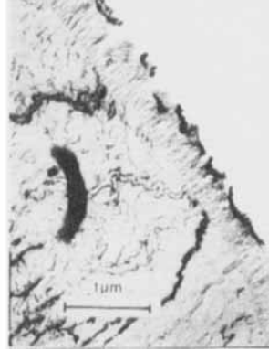
FIGURE 20 Phosphoric acid anodised substrate. Intermittent, cohesive failure.
