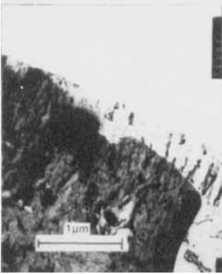
FIGURE 19 Scotchbrite abraded substrate. Essentially adhesive failure.
