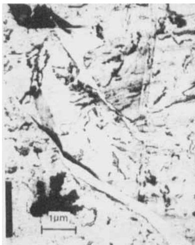
FIGURE 9 Transmission electron micrograph of a section through the aluminium substrate of a grit-blasted bonded joint; it shows the sub-surface cracking.
